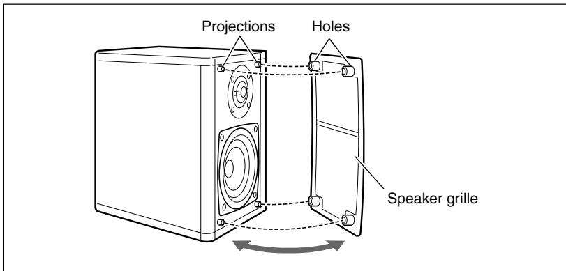
**To remove the speaker grille**, insert your fingers at the top of the speaker grille, then pull towards you. Repeat the procedure at the bottom of the speaker grille.
